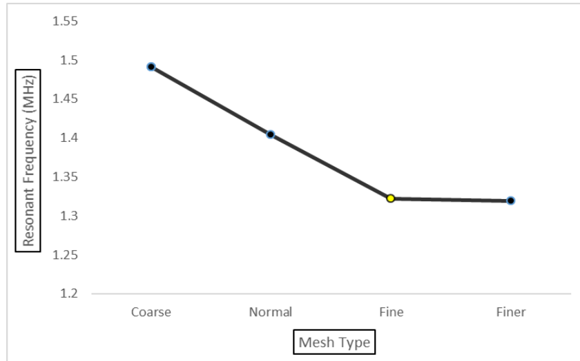
Figure 9 COMSOL simulation results showing the trend of the resonant frequency with the respective mesh type.
